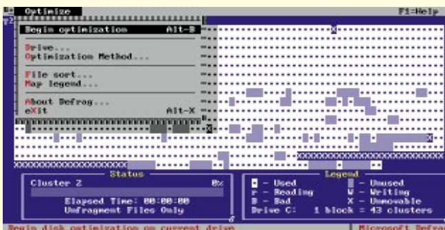
Fig 3 The row of crosses shown here represents the Windows swap file. This should be removed before starting the defragmentation process
